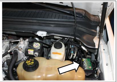
9. Connect the in-cab wiring harness to the control module in the engine bay by plugging in the small eight pin white connector.
