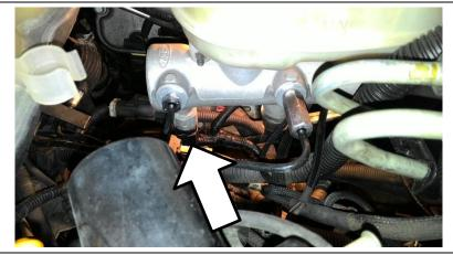
Disconnect the turbo vane actuator. Connect the BD harness to actuator and OE plug.
