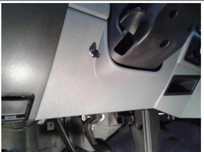
4. Remove the top cover on steering wheel column, locate and disconnect tow/haul connector. Feed the BD harness connectors up from behind the dash and Install the BD harness between the OEM connectors. Replace top cover onto steering column.
